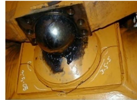
Cracked or broken Ball or Slab.
